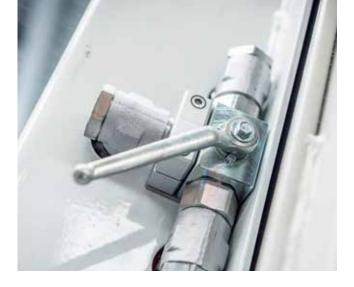
Switching the oil pressure from the tailgate to the floors is done by way of a manually operated ball valve. Robust and malfunction-resistant technology to ensure maximum usability.
