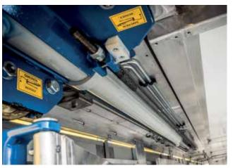
Due to the unique Berdex design, we are able to use just a single dependable cylinder. With fewer moving parts, this system continues to function reliably even with partial wear.
