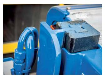
The unique Berdex powered tailgate design with its slide pads features as few moving parts as possible. This ensures dependable usability.
